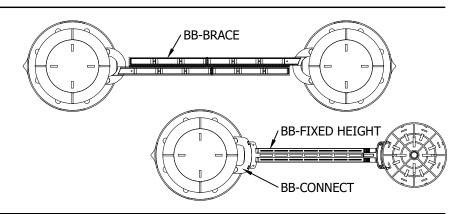
4. LOCK THE BRACING ARMS TOGETHER BY INSERTING BB-LATCHES INTO THE SIDE OF EACH BISON BRACE OR BB-SCREWS INTO THE TOP OF EACH BB-FIXED HEIGHT, AND TWIST 90 DEGREES.
