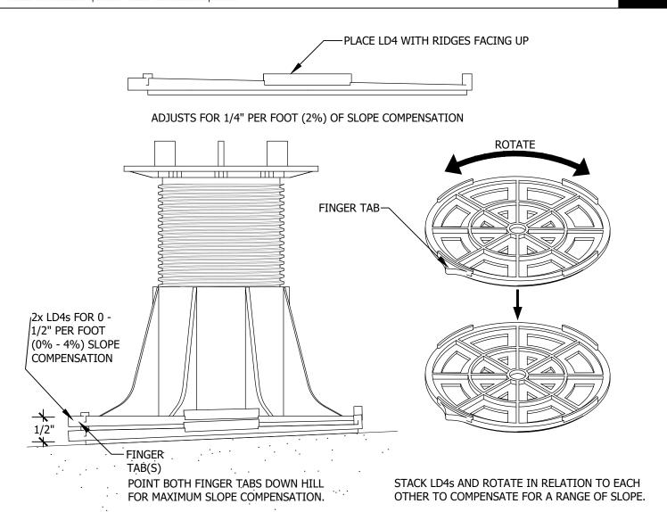
EACH LD4 WILL COMPENSATE FOR 1/4" PER FOOT OF SLOPE (2%) AND ADD 1/4" TO THE OVERALL HEIGHT OF A PEDESTAL. A MAXIMUM OF 4 LD4s MAY BE STACKED BELOW A PEDESTAL IN ORDER TO COMPENSATE FOR SLOPES FROM 0" TO 1" PER FOOT (0-8%).
