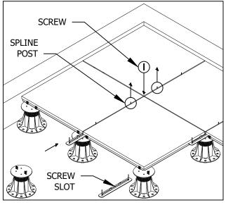
4. SCREW SPLINES INTO CENTER OF PEDESTAL TOPS, AND REMOVE POSTS WITH PLIERS, TAKING CARE NOT TO DAMAGE THE PAVERS. (DO NOT ATTEMPT TO HAMMER THE POSTS)
