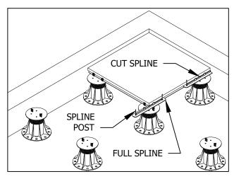
3. USING THE SPLINE POSTS, SLIDE FS-12 SPLINES INTO CHANNEL OVER PEDESTALS. PERIMETER SPLINES IN LINE WITH TRAY CHANNEL SHOULD BE CUT DOWN WITH A SAW AS NEEDED IN ORDER TO CENTER OVER EACH PEDESTAL.
