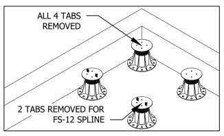
PLACE PEDESTALS AROUND PERIMETER AND REMOVE TABS AS NECESSARY.
