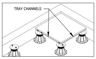
2. PLACE PAVER TRAY ASSEMBLY ON TOP OF PEDESTALS.
