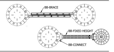
LOCK THE BRACING ARMS TOGETHER BY INSERTING BB-LATCHES INTO THE SIDE OF EACH BISON BRACE OR BB-SCREWS INTO THE TOP OF EACH BB-FIXED HEIGHT, AND TWIST 90 DEGREES.
