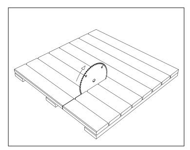
1. AFTER MEASURING, CUT THE TILE TO THE DESIRED SIZE WITH A HIGH QUALITY CARBIDE SAW BLADE. CUT FROM THE TOP AS SHOWN IF USING A HAND SAW OR TURN THE TILE OVER FOR A TABLE SAW.
