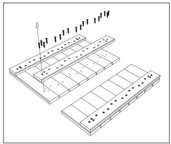
2. AFTER CUTTING, WITH THE TILE UPSIDE DOWN, REMOVE A BOTTOM RUNNER FROM THE PORTION TO BE DISCARDED, BEING CAREFUL TO NOT STRIP THE SCREW HEADS.
