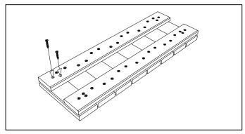
4. AFTER PRE-DRILLING, SCREW THE RUNNER INTO PLACE ON THE PORTION TO BE INSTALLED, RE-USING THE SCREWS REMOVED IN STEP 2.
