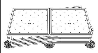
4. REPEATING THE FIRST THREE STEPS, GENTLY LAY EACH NEW PAVER ON TOP OF THE PREVIOUS TRAY, ROTATING AS SHOWN. STACK NO MORE THAN TEN (10x) PAVERS HIGH, AND LET THEM SIT FOR 2 TO 4 HOURS, OR UNTIL THE ADHESIVE HAS CURED, BEFORE HANDLING.
