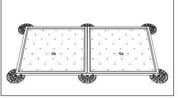
3. PLACE THE ADHESIVE SIDE OF THE TRAYS SQUARELY ONTO THE PAVER, CAREFULLY ALIGNING BY HAND TO MAKE SURE THAT THE TRAY DOES NOT EXTEND BEYOND ANY EDGE OF THE PAVER.
