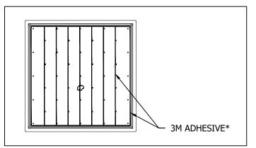
2. RUN A 1/8" DIA. BEAD OF PROVIDED 3M ADHESIVE, OFFSET 1/4" FROM THE TOP OUTER EDGE OF EACH TRAY, AND A 1/8" DIA. BEAD ALONGSIDE EACH LINE OF HOLES AS SHOWN. \*IMPORTANT: FOR PROPER ADHESION AND PERFORMANCE, ADHESIVE MUST BE APPLIED EXACTLY AS SHOWN. TO PREVENT MOISTURE FROM ENTERING BETWEEN PAVER AND TRAY, A CONTINUOUS PERIMETER BEAD OF ADHESIVE MUST BE INSTALLED ALONG THE EDGE OF THE TRAY.
